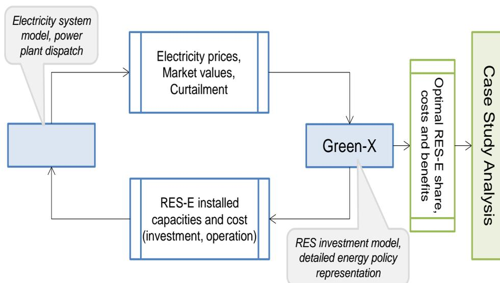
**Figure 1: Model coupling between Enertile (left) and Green-X (right) for a detailed assessment of RES developments in the electricity sector**
