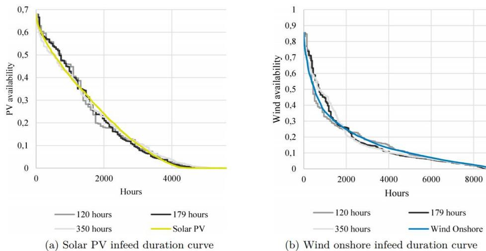
Figure. Original and processed load and infeed duration curves. Source: Gerbaulet & Lorenz 1 (2017)
